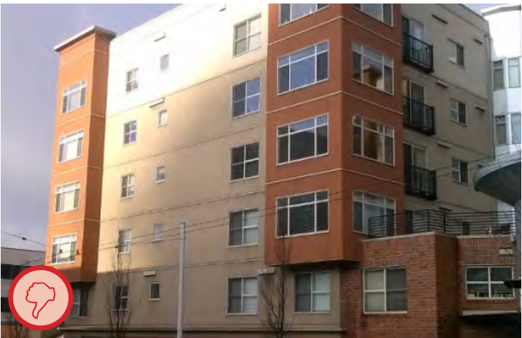
Inappropriate: EIFS is not permitted below the 3rd floor or on street facing building facades
