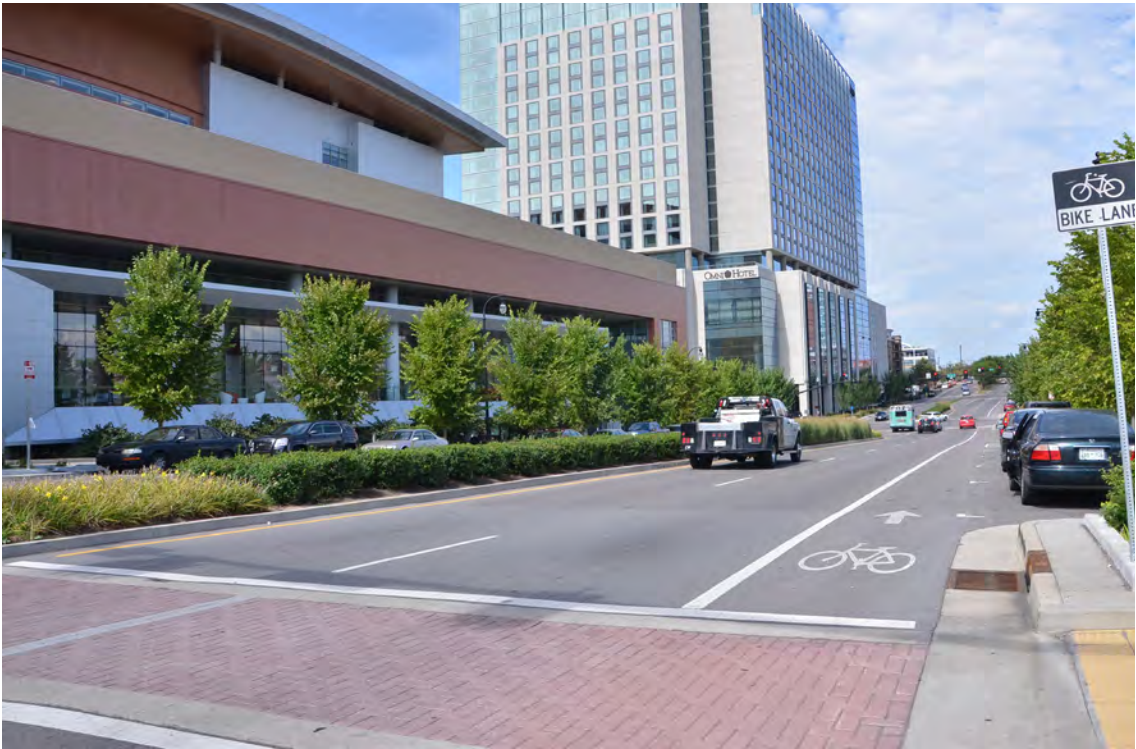
Concrete pavers are used at crosswalks to provide visual cues for vehicles
