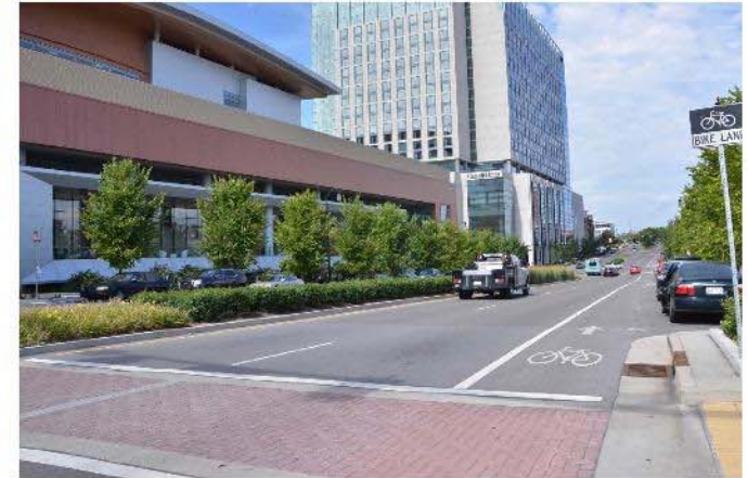
Concrete pavers are used at crosswalks to provide visual cues for vehicles.
